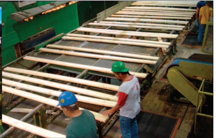
Computer-controlled optimizers scan logs for solutions to the cuts that will yield the highest value.
